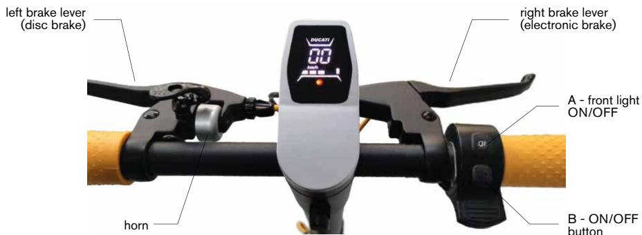
**Power on (B):** Press and hold this button (B) for three seconds to turn the electric scooter on and off.
