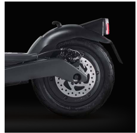
Front and rear disc brake with KERS
